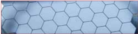
50 µm thick S/S mesh (struts 50 µm x 1.6 mm across flats) Courtesy: Laser Micromachining Ltd
