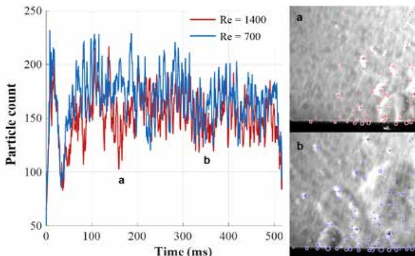
Figure 2: (Left) Total number of particles over scanned area during printing. (Right) Annotated frames of the local minimum count for (a) high flow and (b) low flow. Faster extraction limits laser interaction with airborne particles, thus improving repeatability.
