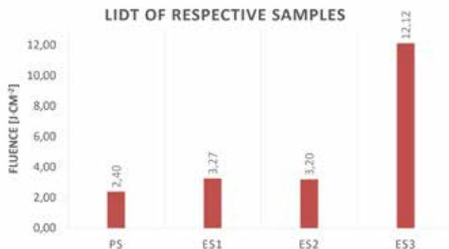
Figure 2: Damage thresholds of tested samples. PS: silver mirror protected with standard SiO<sub>2</sub> layer; ES1: silver mirror protected with standard SiO<sub>2</sub> layer, enhanced with Al<sub>2</sub>O<sub>3</sub> intermediate layer; ES2: silver mirror protected with Al<sub>2</sub>O<sub>3</sub> layer; ES3: silver mirror protected with dielectric multilayer improving the reflectance at 1030 nm and enhanced with Al<sub>2</sub>O<sub>3</sub> intermediate layer.
