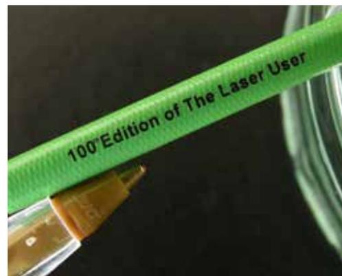
The cover image shows a braided catheter, with a PEBAX outer sheath, metal braid and PTFE inner liner. The outer sheath was removed using short pulsed laser processing. Our thanks to Blueacre Technology for machining the special message in lettering approx. 2 mm high.
