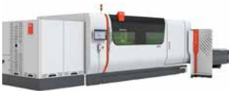
The technological leap from conventional 3-12 kW systems to the new 15 kW level is tremendous. On average, thanks to the 15 kW laser, the cutting speed of the ByStar Fiber increases by up to 50% (when cutting with nitrogen) compared to a 10 kilowatt laser source.
