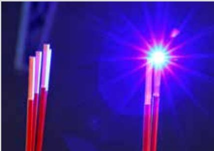
Laserline is optimising its portfolio in the LDMblue high-power diode laser segment with 450 nm wavelength. Primarily developed for copper material processing in the electronics industry, these blue diode lasers are now available in six power levels between 300 and 2,000 watts.
