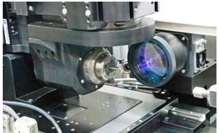
robot was integrated along with other additional components such as an optical measuring system for in-process measurement. The advantage here was that the same Aerotech control system could be used. "This allows us to expand the periphery at any time without having to purchase new control software, for example if we want to integrate a Profibus or an additional piezo axis - we are absolutely open and not restricted at all."
