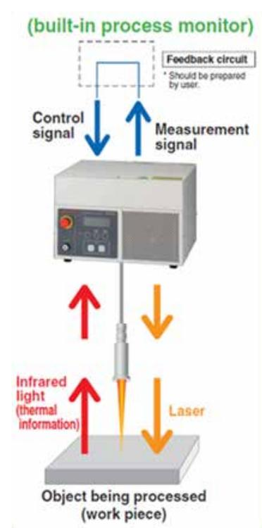
*In the SPOLD system, the temperature is measured coaxially using the same optical fibre as the working laser*
