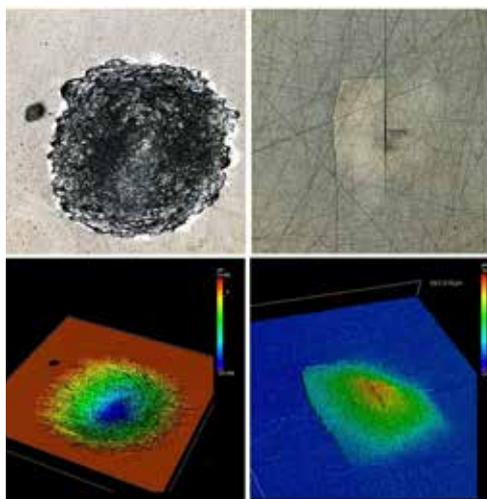
Figure 4. Details of the craters ablated on HgCl crystals with 1,8 ps pulses at 1030 nm. Crystals were prepared in plane 110 (left, damaged at 1 J/cm<sup>2</sup>) and 001 (right, damaged at 5 J/cm<sup>2</sup>)
