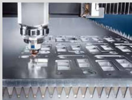
TRUMPF has equipped its latest TruLaser Series 5000 laser cutting machines with a TruDisk 12001 disk laser with 12 kilowatts of laser power.
